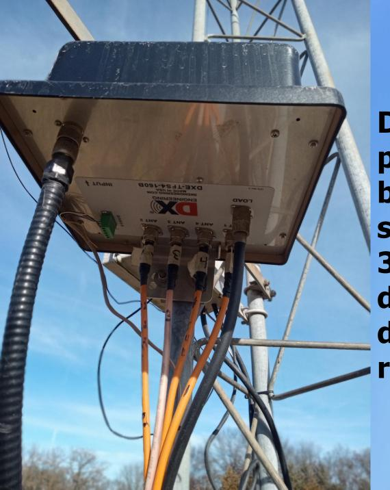
**DX Engineering** phasing/control box for 160m four square - approx. 3% power dumped to dummy load at resonance
